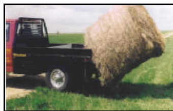
4" x 8" cylinder & spring loaded bale spike locks
